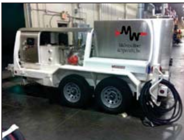
Our mobile testing unit can recertify hoses on-site
